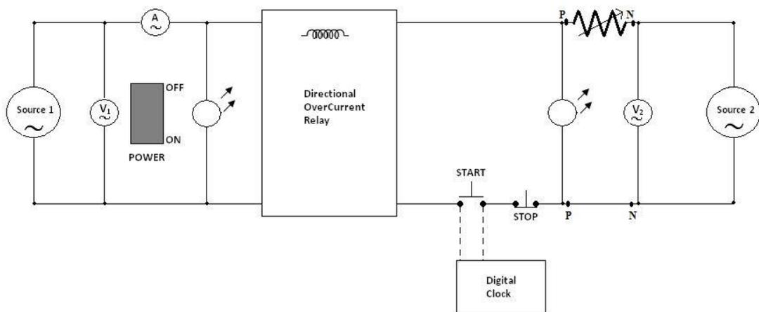
**Fig 7.1:** Over Current Relay
