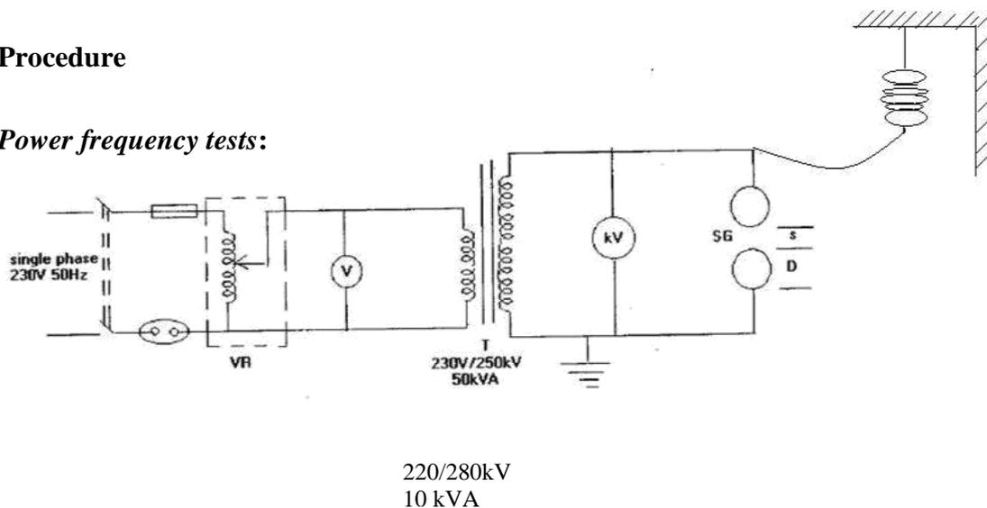
**Figure 6.1:** Circuit Diagram
