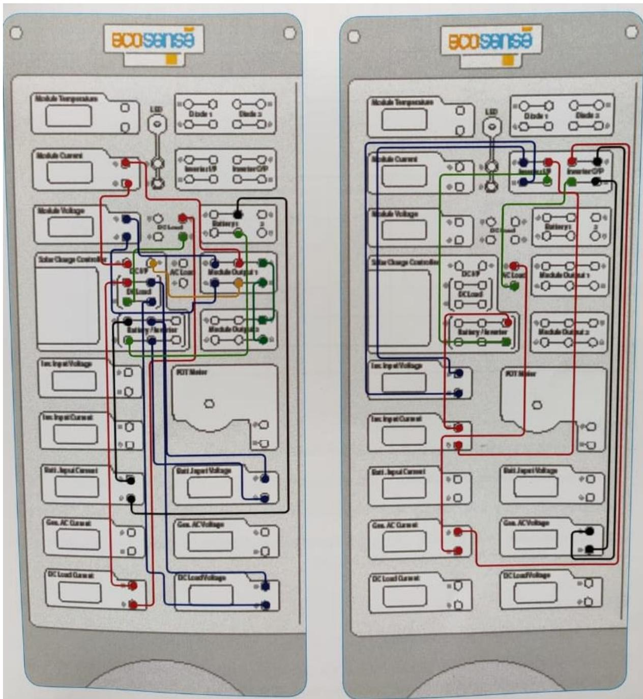
**Fig 13.1:** Control board connections for standalone PV system to supply both AC and DC load
