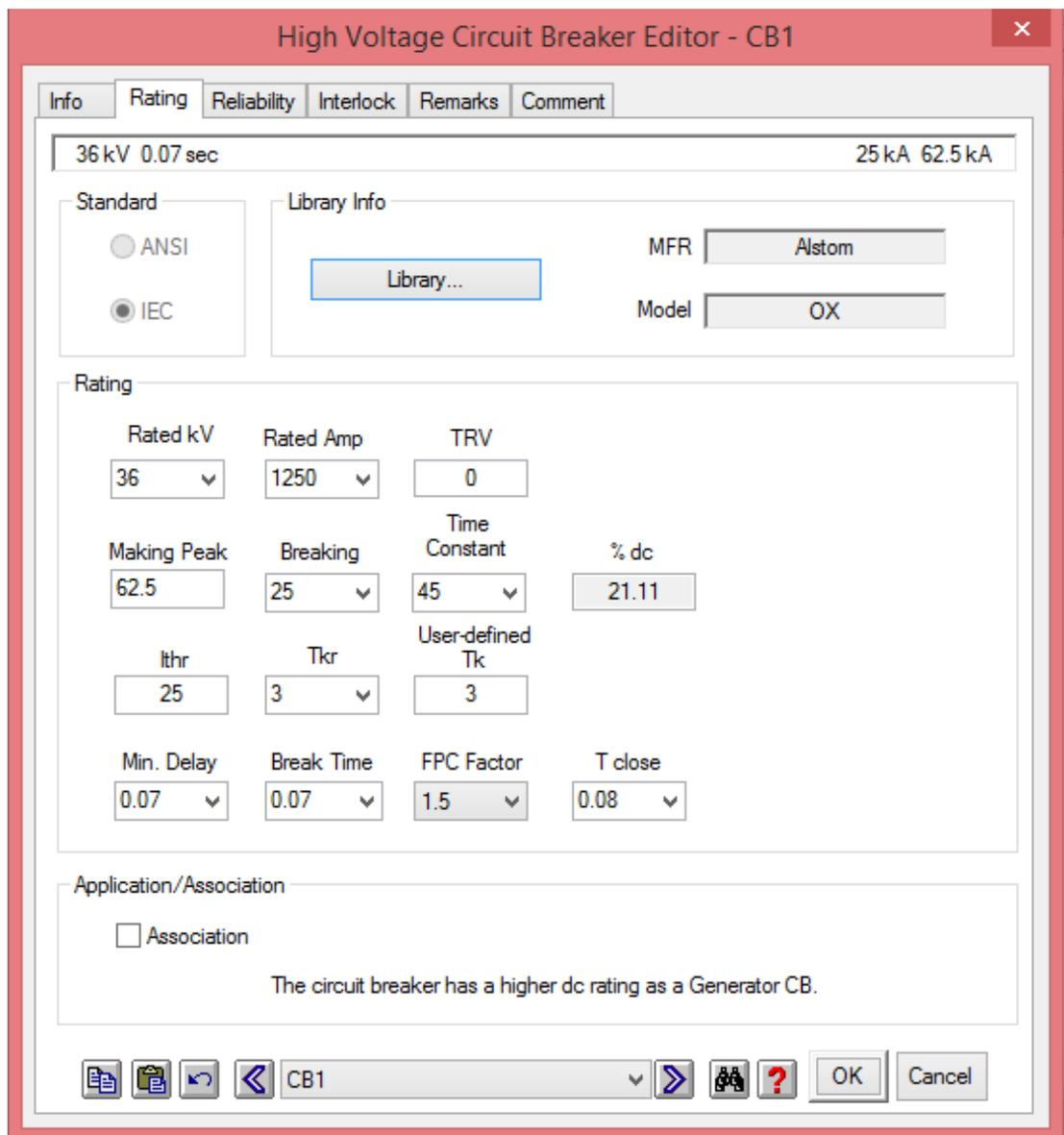
**Fig 16.4:** High Voltage Circuit Breaker Editor
