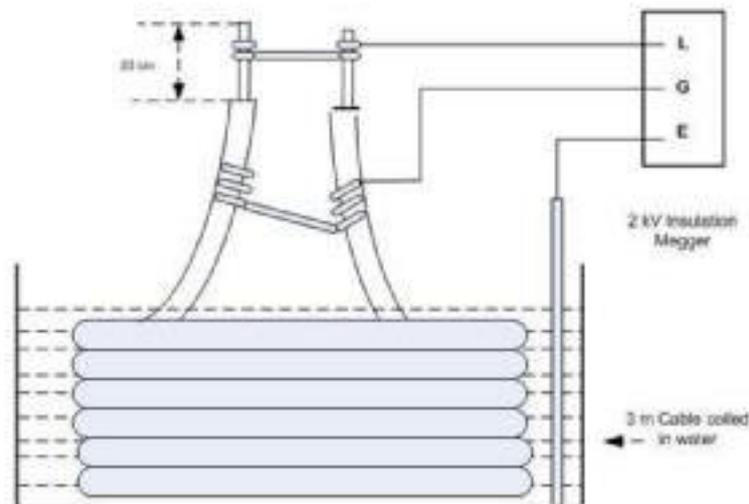
**Fig 8.1:** Insulator Setup
