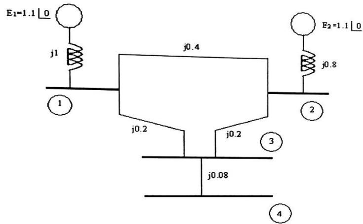
Fig 2.1 Single Line Diagram
