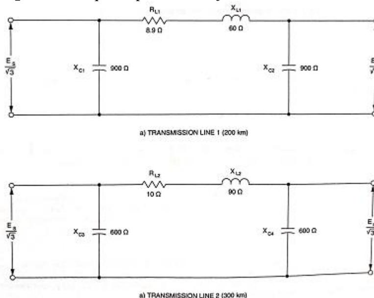
**Fig 17.1** shows the circuit representing one phase of transmission lines 1 and 2 of the demonstrator.
